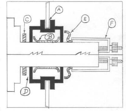
that the tip rest into the depressed area of the "S" washer (Figure 1, item "F").
