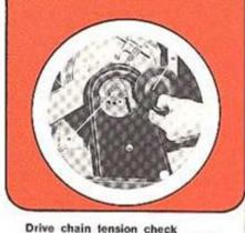
Pull out the chain case cover (m). Move the loose side of the drive chain back and forth. The free play of the chain must be between % " to %".
